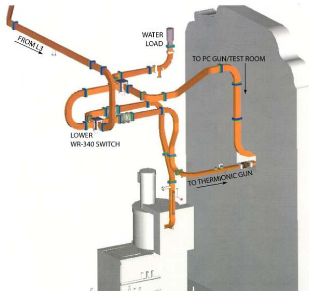
Figure 1: Switching at L1.
