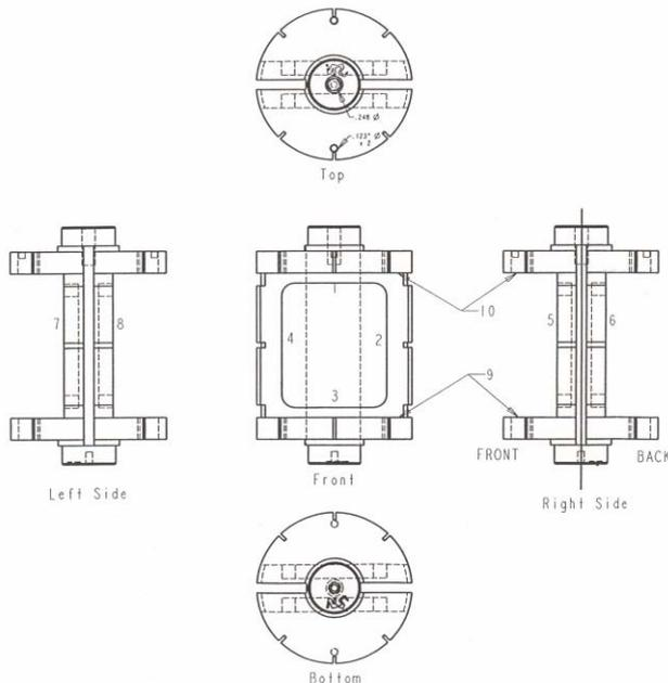
Figure 3: WR-284 rotor edges that are handworked.
