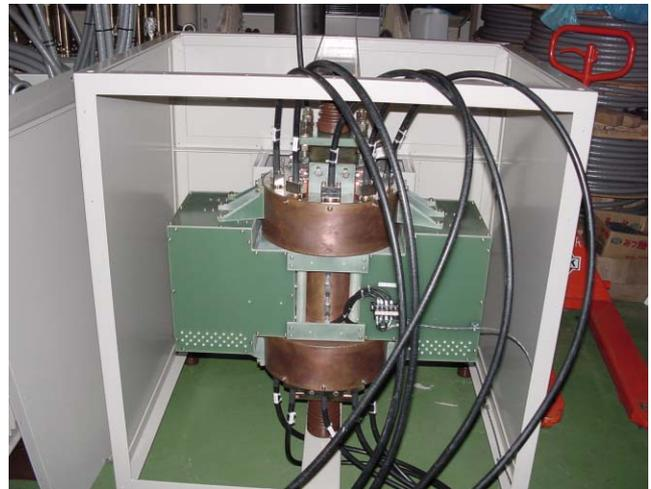
Figure 3: Picture of SI-thyristor module and PFL cable.
