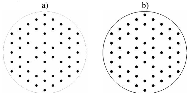
Figure 2: Two lattice configurations for a typical 6-defect, 4<sup>th</sup> order PBG structure.
