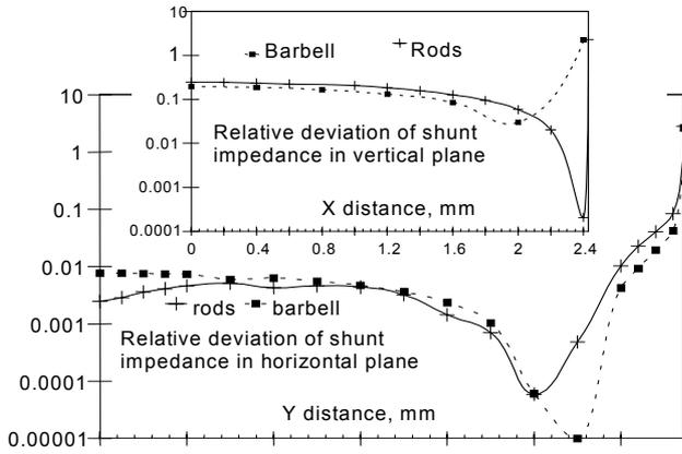
Figure 5: Relative non-flatness of shunt impedance of two planar cavities for the fundamental  $TM_{11}$  mode: barbell (dashed), and one loaded by 2+2 rows of rods (solid line).
