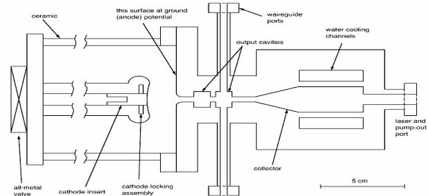
Figure 8: Schematic of a planar, X-band lasertron (“long” dimension into paper).
