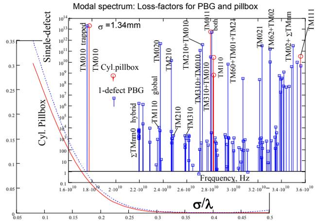
Figure 1: Gaussian bunch TM HOM normalized losses vs rms normalized bunch length (solid line: pillbox cavity; dashed: 1-defect cavity). Inset: spectral losses ( $J\text{-s}/C^2$ ) vs frequency (Hz) for pillbox (circles) and 1-defect cavity (boxes).
