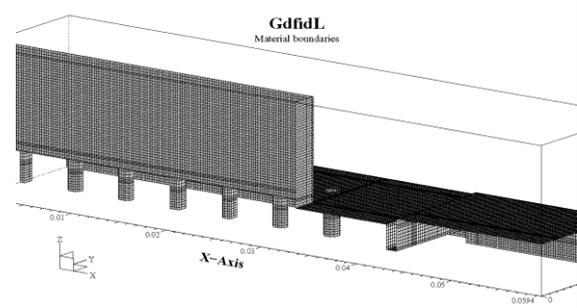
Figure 7: One eighth of a planar PBG structure with 1+1 rows of rods coupled with a WR90 waveguide.
