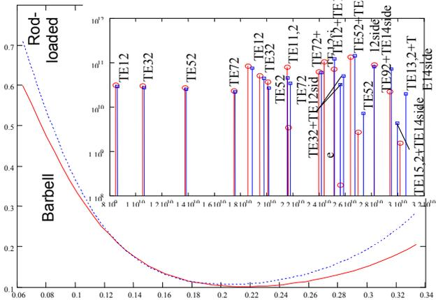
Figure 6: Relative contribution of vertical TE losses of displaced bunch  $\Delta y=0.43\text{mm}$  vs its relative length for barbell and rod-loaded structures. Inset: loss-factor modal spectrum ( $J\text{-s}/C^2$ ) vs frequency (Hz) for vertical dipole symmetrical TE modes in barbell (circles) and rod-loaded (boxes) planar structures at  $\sigma=1.6\text{mm}$ .
