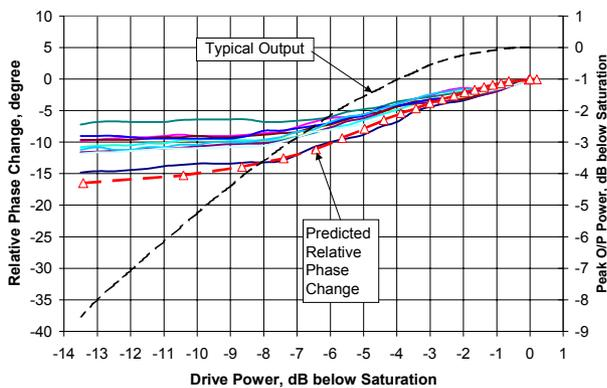
Figure 6: Relative Phase Change vs. Drive Power
