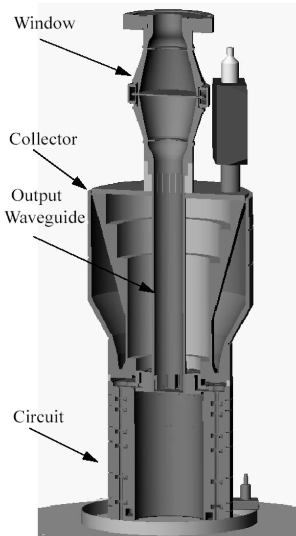
Figure 6: Cross-section of MBK
