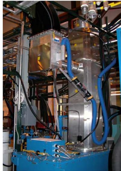
Figure 1: 402.5 MHz, 2.5 MW Klystron
