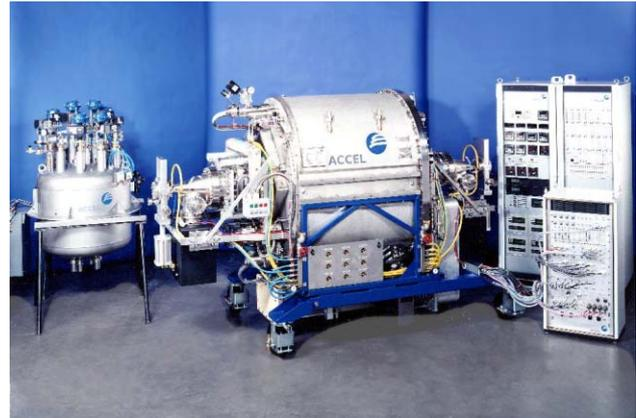
Figure 2: First superconducting accelerator module for the Taiwan Light Source with valve box (left) and SRF electronics (right)
