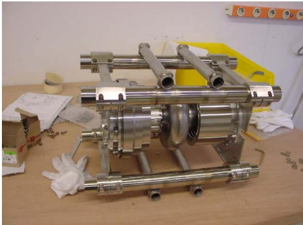
Figure 8: Landau Cavity in handling frame
