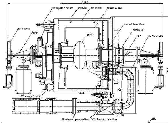
Figure 1: Schematic view of the superconducting module
