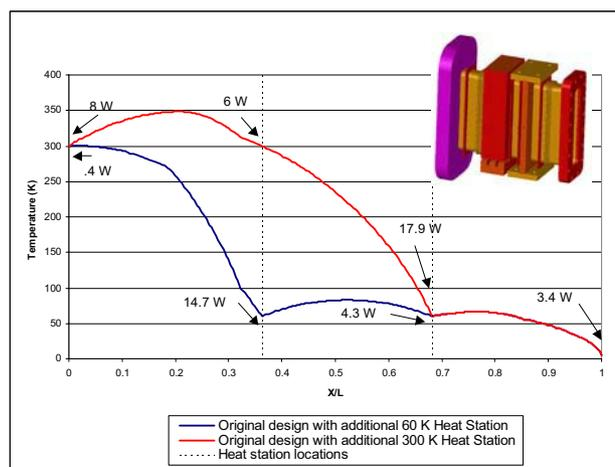
Figure 2: 13 kW Waveguide Thermal Profile
