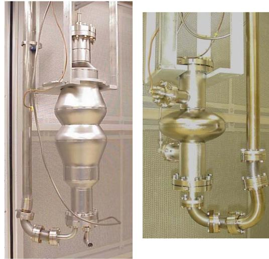
Figure 4: 2-cells cavity (left) and CEBAF single cell (right) on the vertical test stand.
