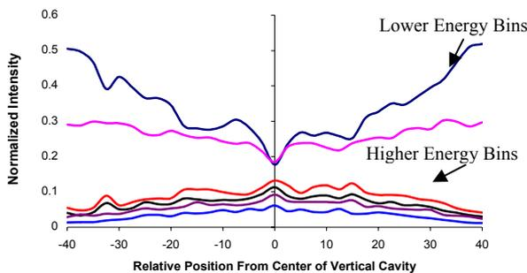
Figure 3: Binned and normalized x-ray energy spectrum from a  $\beta=0.47$  single cell cavity measured through 0.8m of concrete [2]. The peak electric field level in the cavity varied between 38.22-38.48MV/m.
