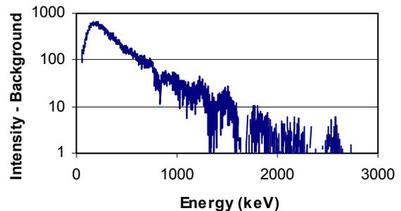
Figure 2: A typical x-ray energy spectrum from a  $\beta=0.47$  single cell cavity measured on top of the Dewar lid [2]. The peak electric field level in the cavity was 21.88MV/m and the maximum electron kinetic energy 1200keV.
