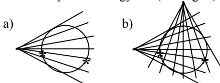
Figure 4: (a) Angular view in one position showing two x-ray sources. (b) An additional view will provide three dimensional information and resolve multiple sources.
