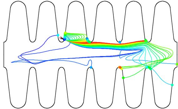
Figure 5: Field emission simulation. The electron emission site is near the iris in the third cell. Primary clusters of electron impact, or primary x-ray emission sources, are seen in the third and fifth cells [3].
