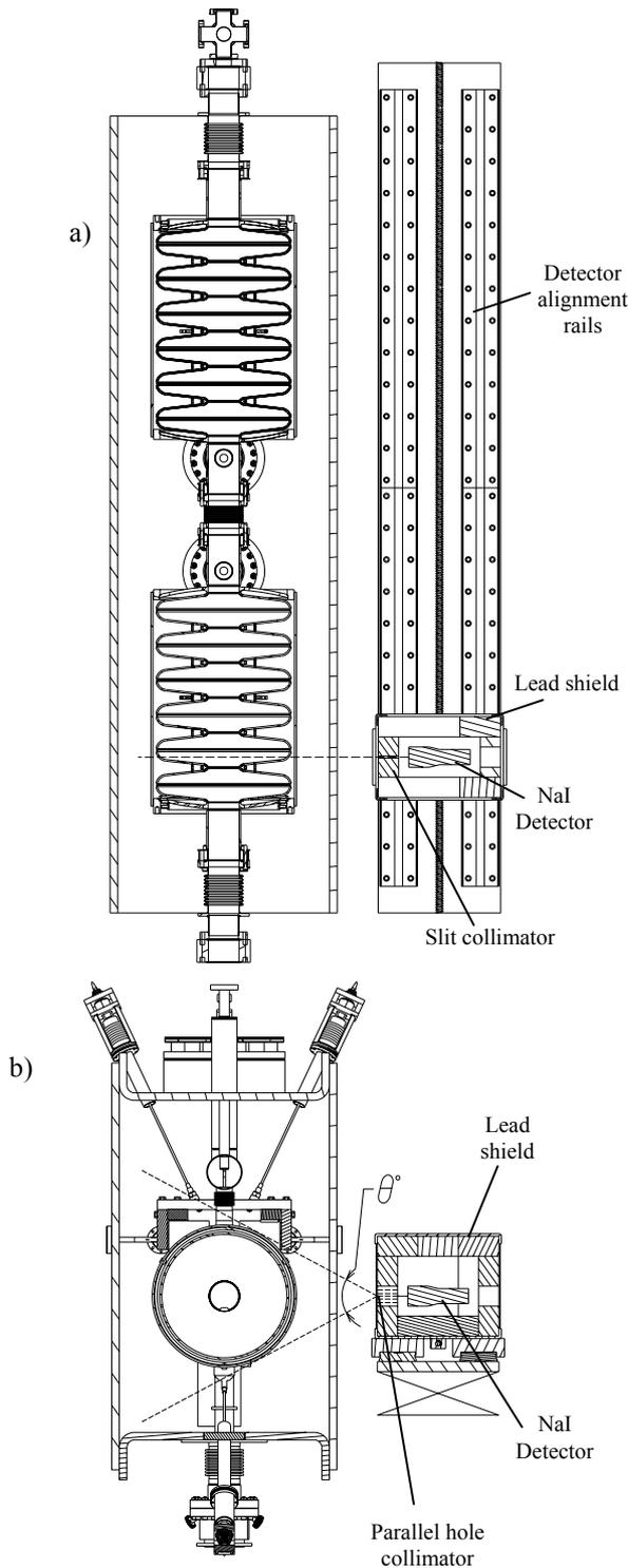
Figure 1: (a) Top view of slit collimator scanning the cryomodule in the horizontal direction [4,5]. (b) End view of parallel hole collimator scanning the diameter of the cavity [4,5].
