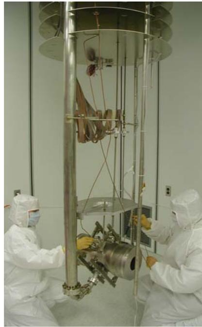
Figure 4: Spoke cavity on the dunking Dewar insert.
