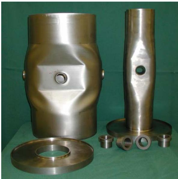
Figure 3: Niobium parts before final welding.
