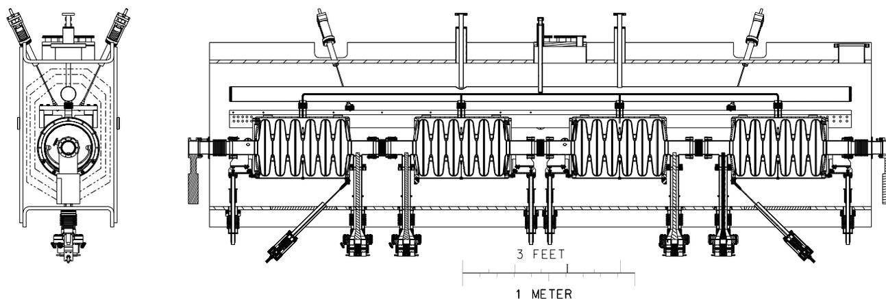
**Figure 1.** RIA Cryomodule with four  $\beta=0.47$  elliptical cavities (side and end view).
