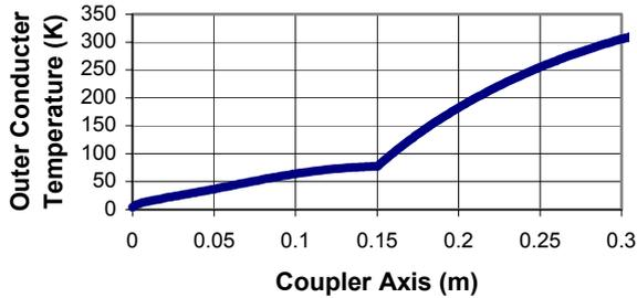
**Figure 3.** Temperature profile along outer conductor of the power coupler.
