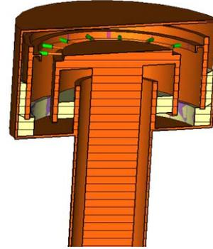
Fig 4. Drawing of a distributed element approach for a high-frequency VCX. The light components are ceramics acting as capacitors, and the PIN diodes are the circumferentially distributed cylinders. The region where the PINs are located would be filled with liquid nitrogen.
