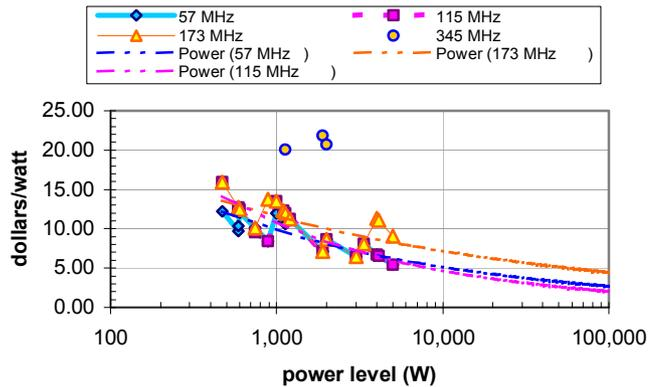
Fig 3. Cost data expressed in dollars per Watt as a function of power level. Power-function fits show how the data scales to higher power values consistent with \$3–5 /Watt.
