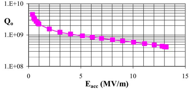
Figure 4:  $Q_0$ - $E_{acc}$  curve at 2 K of the Q-degraded cavity EZ02. This cavity was held at 100 K for a total 180 hours. The  $Q_0$  at the lowest measured  $E_{acc}=0.37$  MV/m was  $4.54E9$ , which was still lower than the initial value of  $\sim 6E9$  of the non-degraded cavity.
