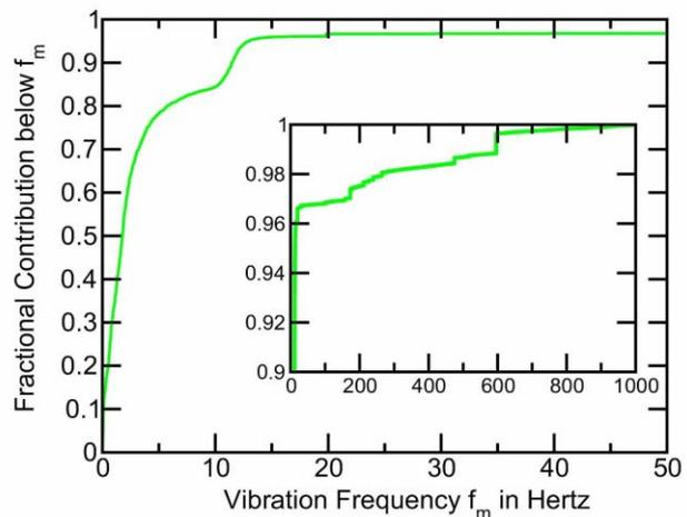
Figure 4 Fractional contribution to the total cavity shake from vibrations at and below the frequency  $f_m$ . The inset shows the same curve extended to vibrational frequencies up to 1 kHz. The result is based on the same data as used for Figure 3.
