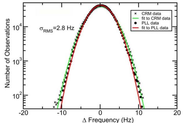
Figure 1. Two methods for measuring rf eigenfrequency shifts (see text) in the two-cell spoke cavity due to microphonics.
