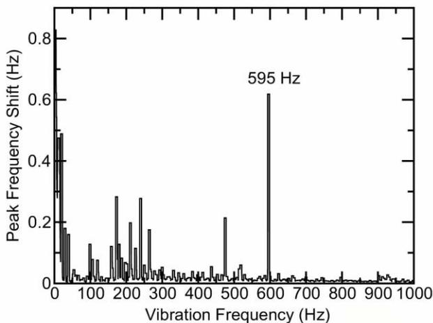
Figure 3. Frequency spectrum for vibrations in the two-cell spoke cavity running cw at  $E_{ACC}=7$  MV/m.
