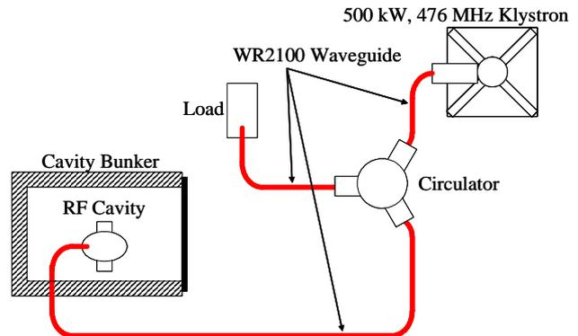
Figure 1 RF Cavity Processing Test Facility Layout
