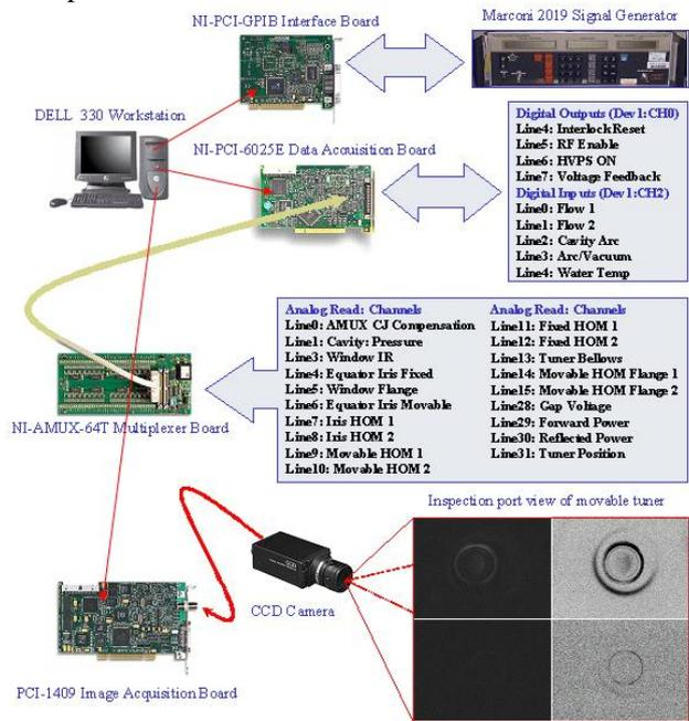
Figure 2 Analog and Digital Diagnostics and Controls
