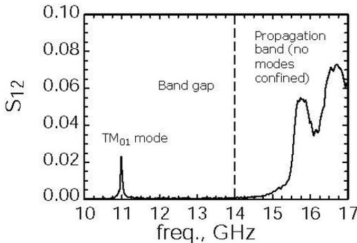
Fig. 4: The transmission curve for a PBG resonator.
