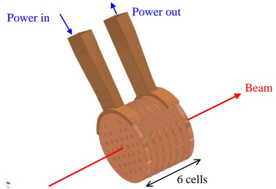
Fig. 5: A 6-cell  $2\pi/3$  PBG accelerator structure
