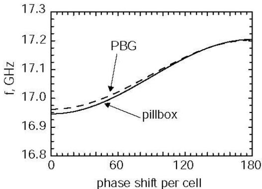
Fig. 7: A comparison of dispersion characteristics for PBG and pillbox accelerator cells with similar irises.
