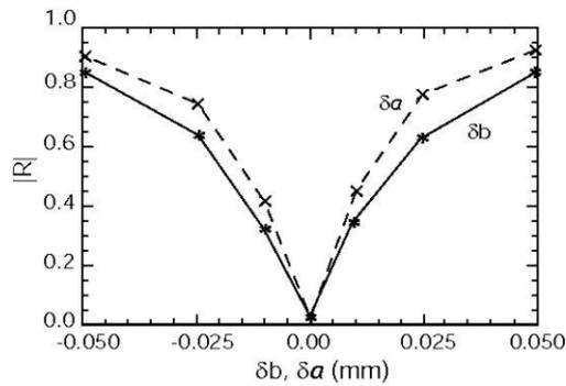
Fig. 6: The reflection from the PBG coupler as a function of deviation of the rods radii (a) and spacing (b) from those given in Table 2.
