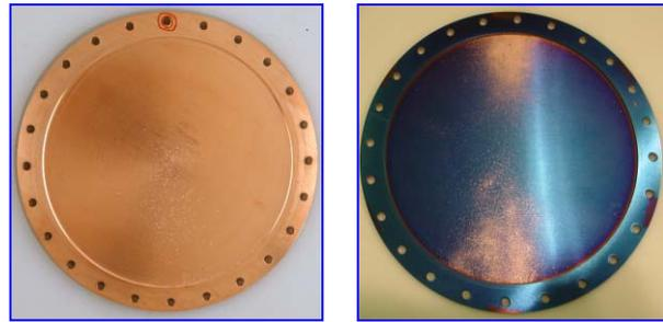
Figure 3: Cu window (left) and Be window (right) after RF conditioning with magnetic field. Deposited Cu particles on the Be window can clearly be seen.
