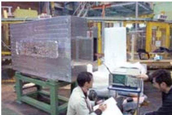
Figure 4: Photograph of the 150MeV FFAG cavity. (After a vacuum duct with a ceramic gap was inserted)
