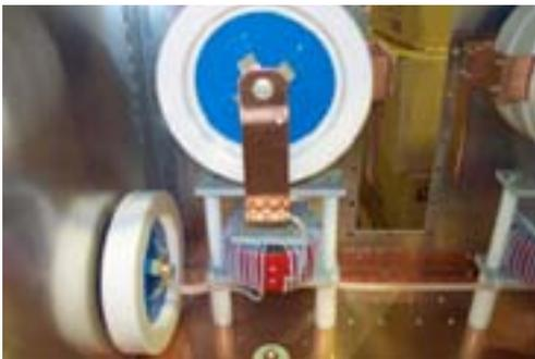
Figure 8: Photograph of the output circuit in the rf power amplifier. An RFC and dc cut capacitor are connected by the large sized cooper bus bar. RFC is winding on three pieces of toroidal cores.
