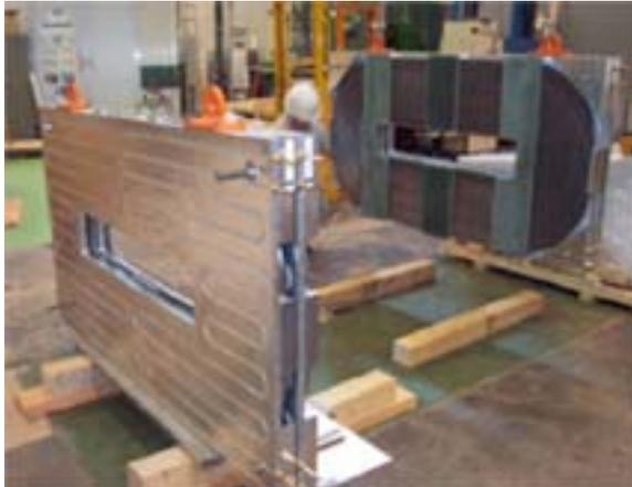
Figure 3: Photograph of cooling plates and MA cores
