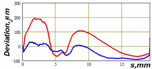
Fig.4. Deviation from design shape after drawing+coining (red), and following annealing+coining+drawing (blue).
