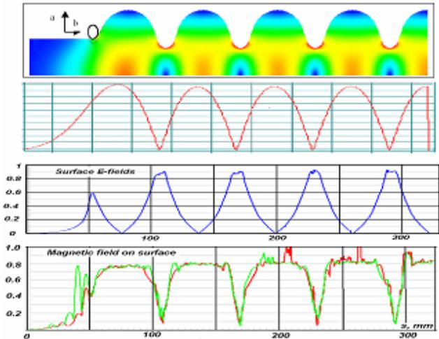
Fig.1. E-field (from the top: in cavity, on axis and on surface) and H-field on surface (bottom). HFSS.
