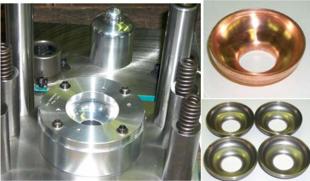
Fig.3. Tooling. Copper and niobium half-cells.
