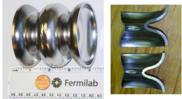
Fig.5. Welded dumbbells
