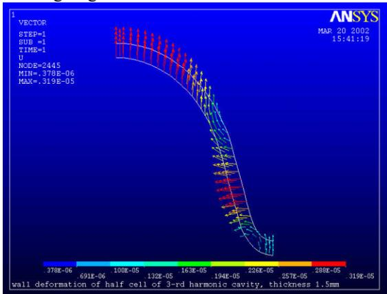
Fig.2. Distribution of surface displacement.
