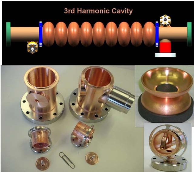
Fig.7. Cavity, end-tubes, dumbbells and HOM couplers.
