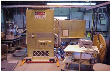
Cavity and the PA under test
