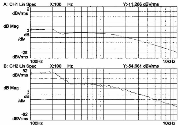
Figure 3: Phase shift and current response plots. The upper trace is tuner bias current, and the lower trace is relative rf phase shift.
