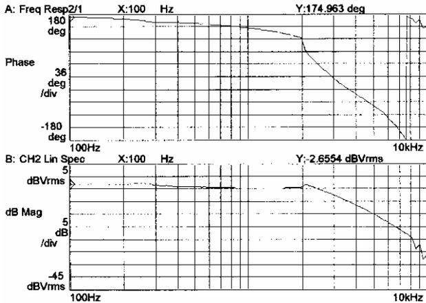
Figure 4: Cavity tuning closed-loop frequency response.
