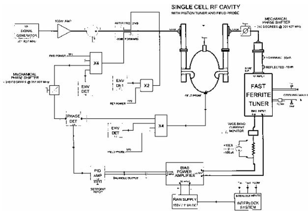
Figure 2: Schematic of test setup.
