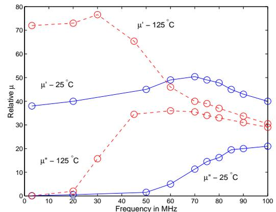
Figure 2: Complex permeability as a function of frequency for both room temperature and 125°C.
