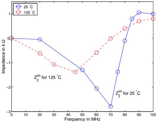
Figure 4: Imaginary longitudinal impedance for one inductive insert at room temperature and 125°C.
