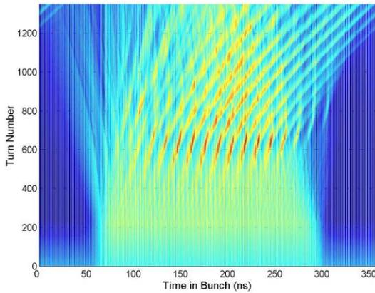
Figure 7: Experimental time mode evolution at room temperature (color).
