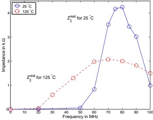
Figure 3: Real longitudinal impedance for one inductive insert at room temperature and 125°C.
