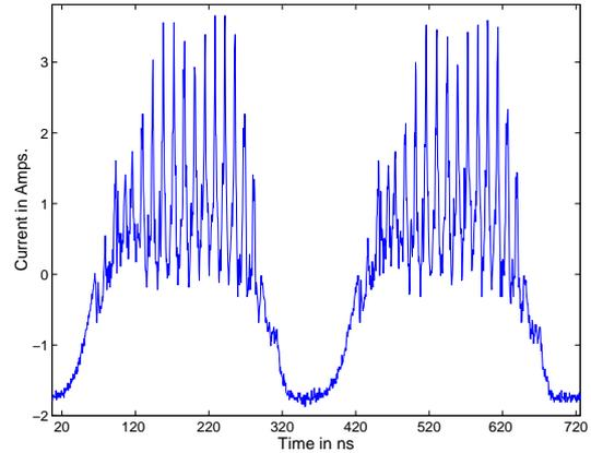
Figure 1: Longitudinal instability caused by the inductive inserts at room temperature.
