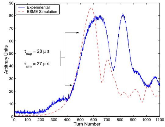
Figure 5: Experimental and ESME growth of the longitudinal instability at room temperature.
