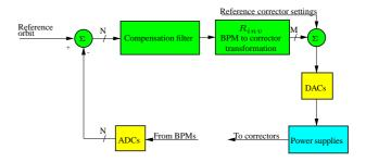
Figure 6: Block diagram of a global orbit feedback system
