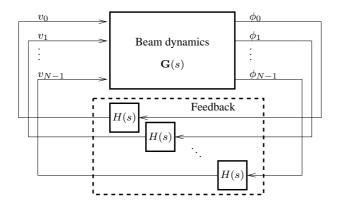
Figure 3: Block diagram of the beam and the bunch-bybunch feedback system
