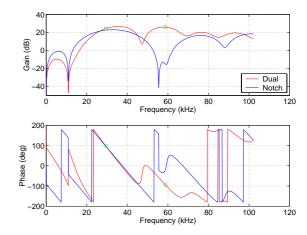
Figure 4: Magnitude (top) and phase (bottom) responses of a dual-peak and peak-notch filters used in control and study of quadrupole instabilities in DA $\Phi$ NE  $e^-$  ring
