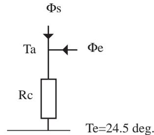
Figure 6: thermal model of the in-vacuum undulator
