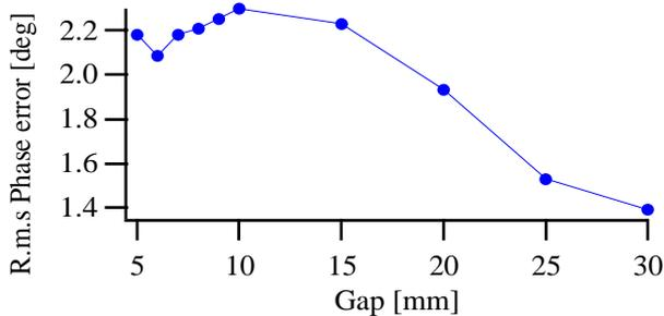
Figure 4: R.m.s phase error as a function of gap for the ID30 U23 device.
