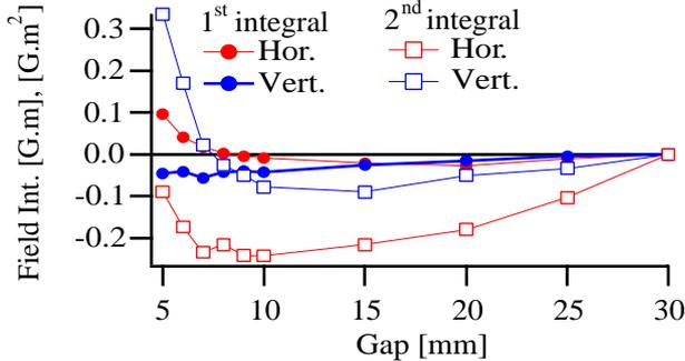
Figure 3: On-axis first and second field integrals component as functions of gap for the in-vacuum undulator ID30 U23.
