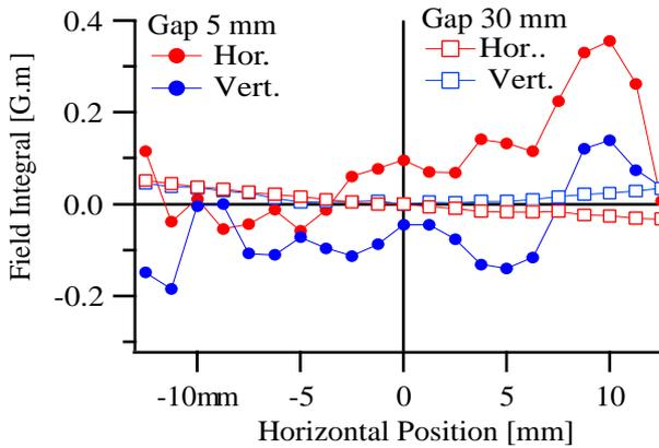
Figure 2: Field integral components versus horizontal position for the in-vacuum undulator ID30 U23 at gaps 5 mm (circular markers) and 30 mm (square markers).
