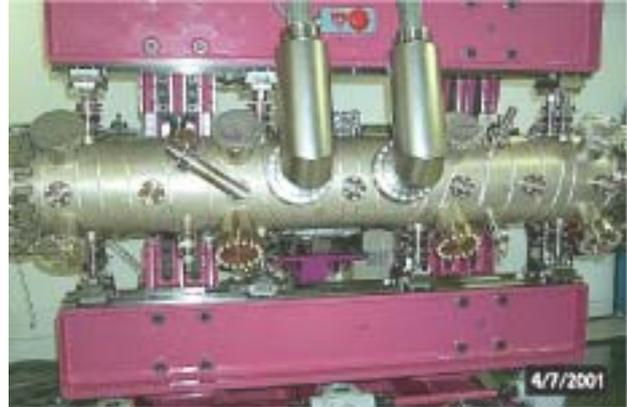
Figure 1: Standard 2 m long ESRF in-vacuum undulator ready for installation
