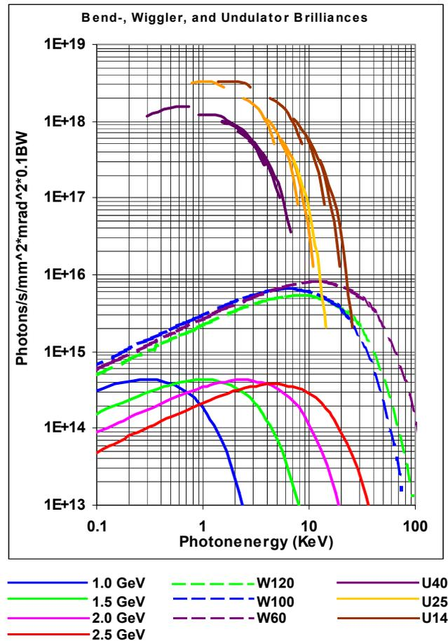
Figure 4: Brilliance of the synchrotron radiation emitted from the stored beam in the bending, wigglers and undulators.
