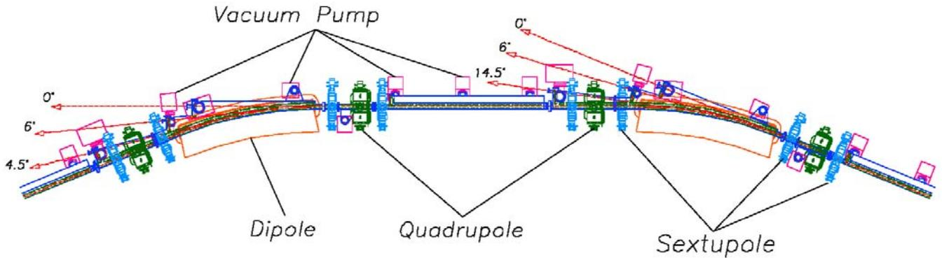
Figure 2: Arrangements of magnets within one unit cell of the storage ring SESAME.
