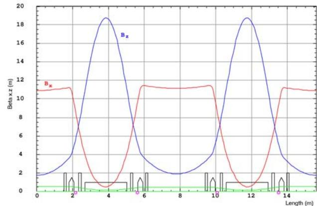
Figure 1: Optical functions of SESAME lattice, The green line represents dispersion, the pink circles represent the BPMs, while the correctors will be inside the sextupoles.
