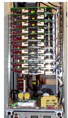
Figure 6: 15-kV IGBT kicker pulser.
