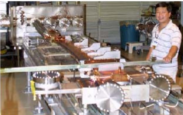
Figure 4: BM1 chamber after bake-out.
