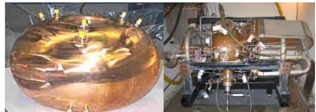
Figure 5: RF cavity body plated with leaky "brightened" copper (left) and leak-tight pure copper (right).
