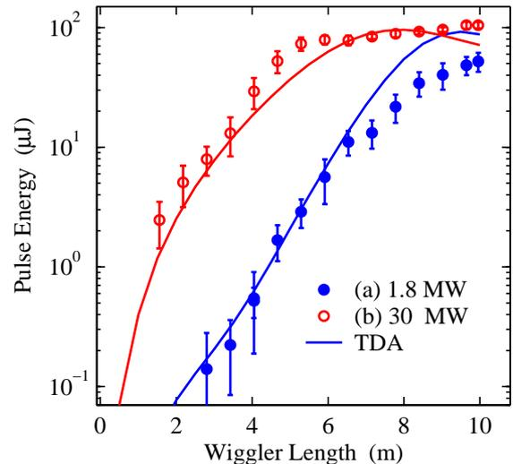
FIG. 2: Pulse energy vs. distance for two values of the input seed laser power: (a) 1.8 MW and (b) 30 MW. The solid curves are TDA simulation results.
