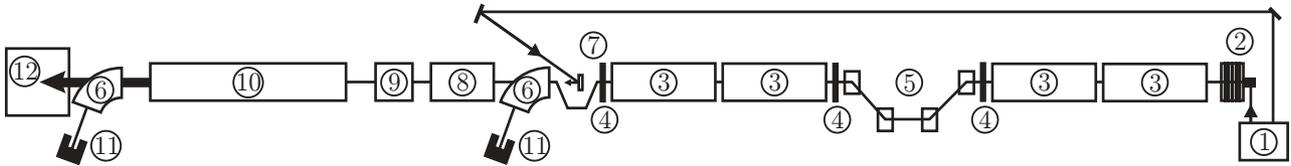
FIG.1: The NLS DUV-FEL layout: 1-gun and seed laser system, 2-RF gun, 3-linac tanks, 4-focusing triplets, 5-magnetic chicane, 6-spectrometer dipoles, 7-seed laser mirror, 8-modulator, 9-dispersive section, 10-radiator (NISUS), 11-beam dumps, 12-FEL measurement area.
