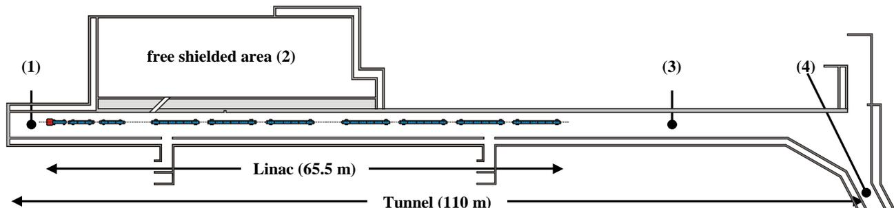
Figure 2: Overview of the existing linac tunnel. The marked areas are: location of a RF photo-injector test stand (1), a shielded area for the driving laser (2), and free area to facilitate the installation of an undulator and moving of accelerator modules (3). The area on the bottom right (4) leads to the injection point of the storage ring. The klystron area is located above the linac tunnel.
