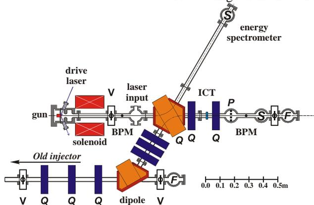
Figure 3: Schematic layout of the injector: (F) faraday cup, (P) pepper pot, (Q) quadrupoles, (S) screens, and (V) vacuum valves. The Faraday cup on the right indicates the position of the first accelerator cavity. The beam-line at the bottom enables use of the present thermionic gun.
