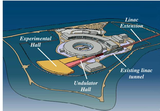
Figure 1: Overview of the ELETTRA laboratory-site after completion of the FERMI project. In the center and top are the buildings in place today. On the left, the undulator hall and the experimental hall are an extension of the existing linac tunnel. The linac extension on the right permits an extension of the spectral range from 10 to 1.2 nm.
