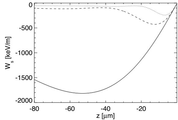
Figure 1: Wake potential for copper, steel and graphite vacuum chambers (dotted, dashed and solid line, respectively) and a 3.4 kA step profile.
