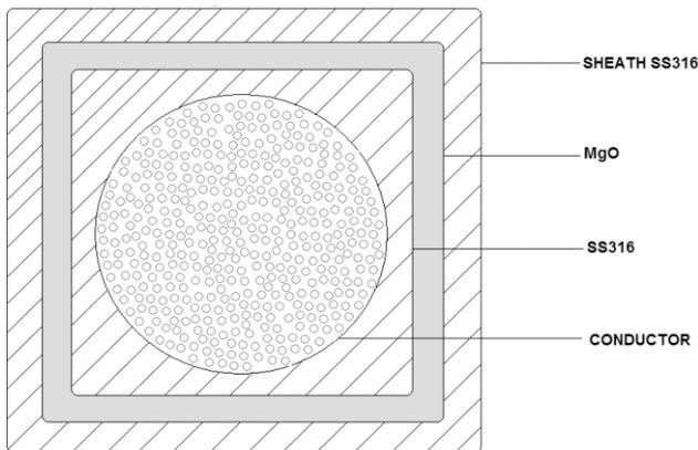
Figure 4: Metal oxide insulated CICC.
