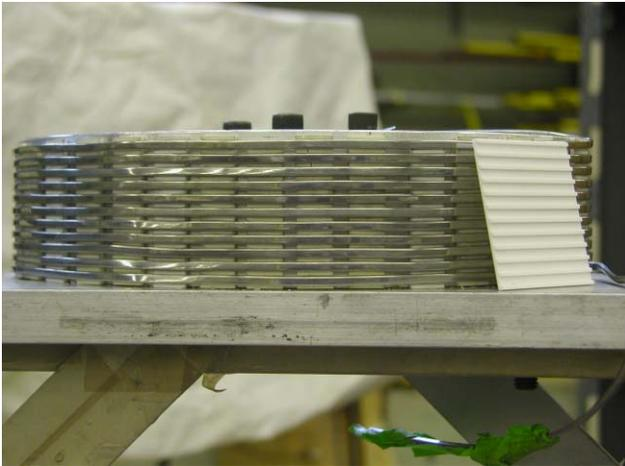
Figure 1: All-inorganic, cryostable test coil.
