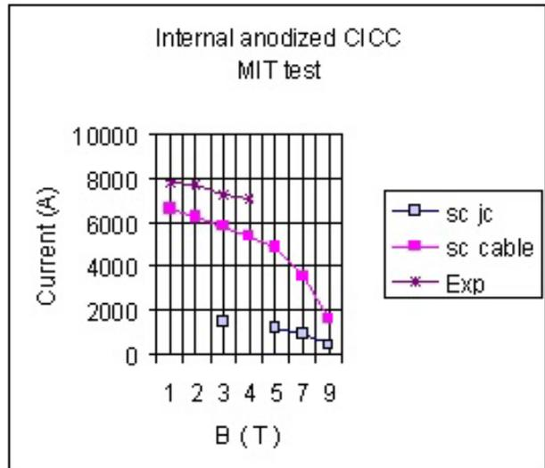
Figure 3: Test results. The curve labeled “sc jc” is the current density in the superconductor in A/mm
