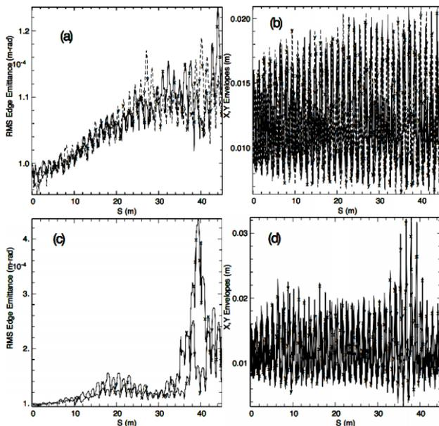
Fig. 3. x-y emittances (a,c) and envelopes (b,d) for randomly modulated density about 5% (a,b) and 10% (c,d) relative electron density
