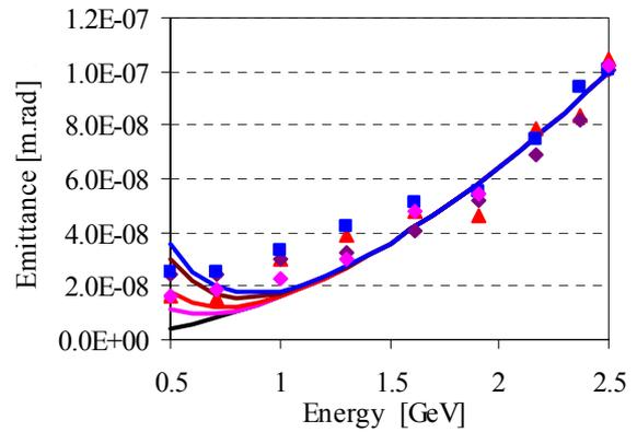
Figure 7: Intrabeam scattering calculations (lines) and emittances calculated from beam size measurements (points). For 0.04 (pink), 0.2 (red), 1 (violet) and 2 (blue) mA per bunch. Black line: natural emittance.
