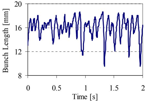
Figure 6: Bunch length vs. time of a 15 mA beam excited by a longitudinal mode at 500 MeV.
