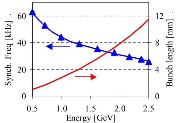
Figure 1: Synchrotron frequency (measurement: points, and fit: line) and bunch length calculation.
