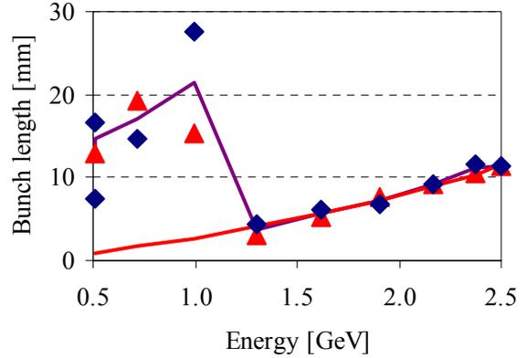
Figure 4: Bunch length as a function of beam energy for a 1 mA beam.
