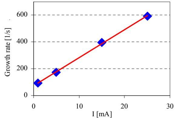
Figure 5: Growth rate of the longitudinal instability as a function of the beam current.
