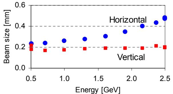
Figure 8: Beam size as a function of the energy for a 2 mA per bunch beam (50 mA in 25 bunches).
