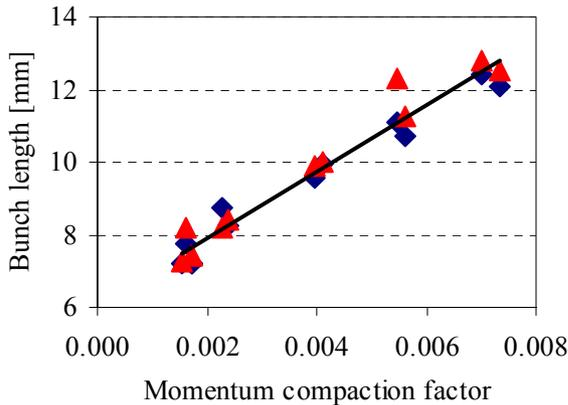
Figure 3: Bunch length as a function of the momentum compaction factor
