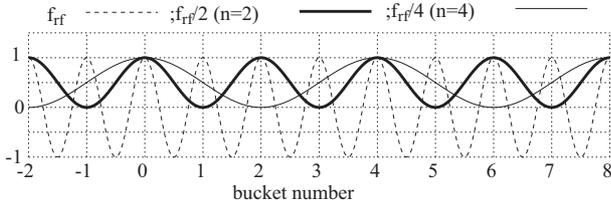
Figure 2: sinusoidal signals with DC offset at the frequency of  $f_{rf}$  divided by an integer  $n$
