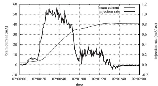
Figure 1: Typical change of beam current and injection rate during injection.
