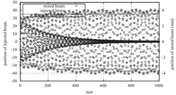
Figure 7: Result of numerical simulation assuming a wake potential
