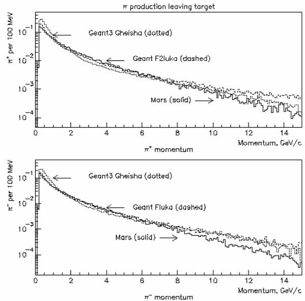
Figure 2:  $\pi^+$  (upper) and  $\pi^-$  (lower) production from carbon target. Rates are per 100 MeV per  $10^5$  protons on target.
