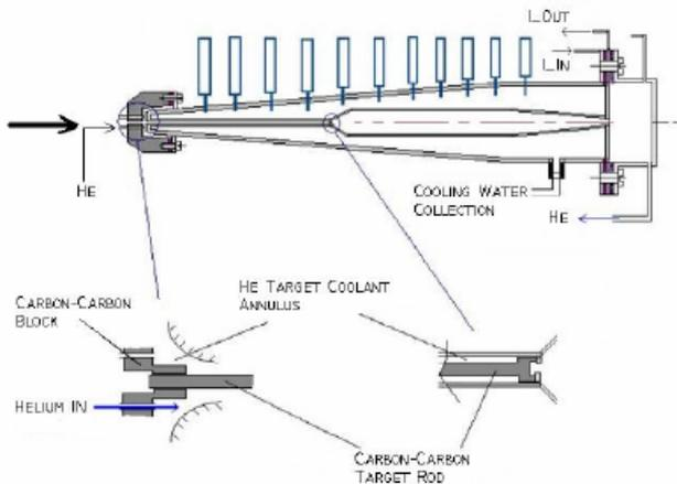
Figure 1: Sketch of First Horn with target inserted.
