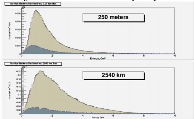
Figure 3: Neutrino Flux Distributions at the close (upper) and far (lower) detectors. Each plot shows the dominant  $\nu_\mu$  with the  $\nu_e$  distribution superimposed in a darker color. The  $\nu_e$  flux is scaled by a factor of 20 to be visible.
