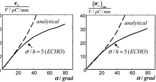
Fig. 3. Transverse wake dependence on collimator angle.
