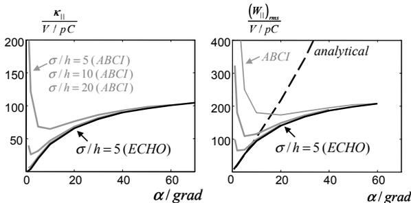
Fig. 2. Longitudinal wake dependence on collimator angle.
