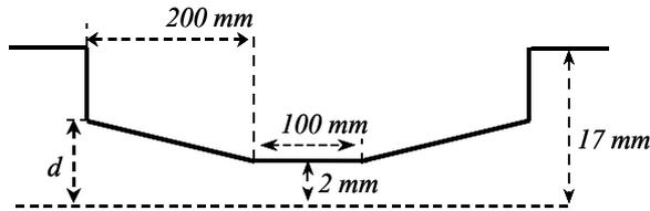
Fig. 5. Geometry of the TESLA TTF2 “step+taper” collimator.
