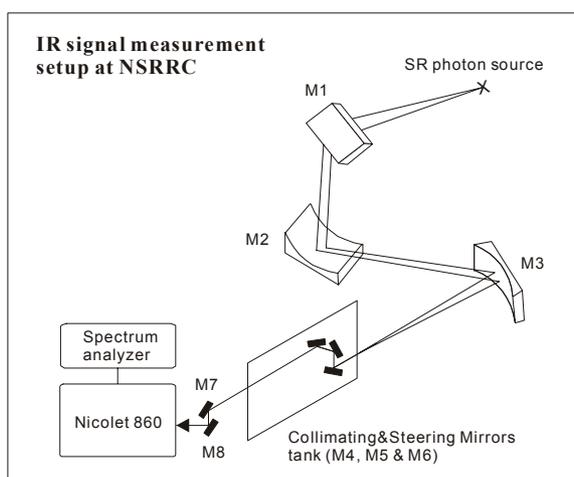
Figure 2: Schematic Diagram of Optical Layout of IR beamline at NSRRC
