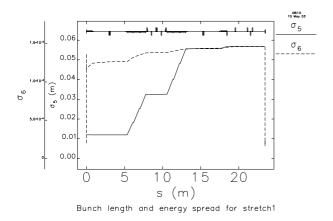
Figure 4: The evolution of the rms bunch length  $\sigma_5$  and the energy spread  $\sigma_6$  in the beam line.
