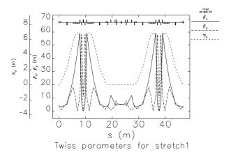
Figure 1: The  $\beta_x$ ,  $\beta_y$  and  $\eta_x$  in the beam line.
