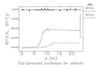
Figure 3: The evolution of the emittance  $\epsilon_{n(x,y)}$  growth in the beam line.
