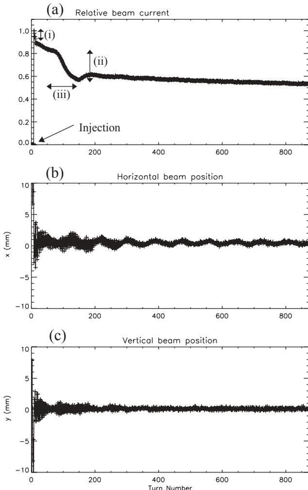
Figures 5: Coherent oscillation of the injected beam:(a) shows the turn-by-turn relative beam current, (b) the horizontal beam position and (c) the vertical one. The horizontal axis indicates the turn number from the injection.
