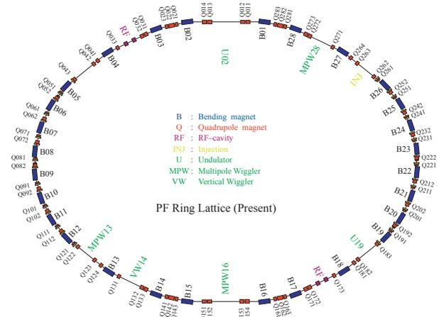
Figure 1: Lattice configuration of PF ring.
