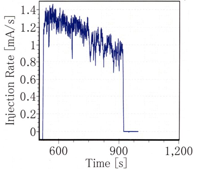
Figure 6: Typical injection history is shown when beam was stored from a current of 0 mA to 450mA .
