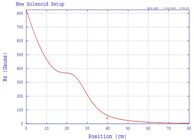
Figure 2: Bz from new solenoid setup
