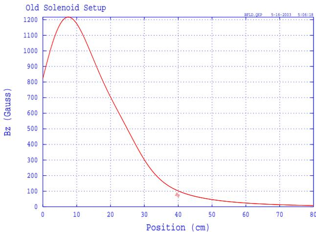
Figure 1: Bz from old solenoid setup
