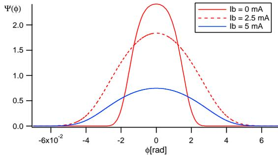
Figure 4: Longitudinal distribution for various bunch intensities in the potential well regime – Prediction with a harmonic RF system at the ESRF tuned for optimum bunch lengthening.
