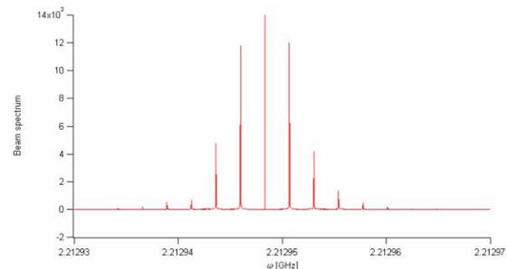
Figure 1: Beam spectrum for  $V_h = V_{h,opt}$  around the main RF frequency.
