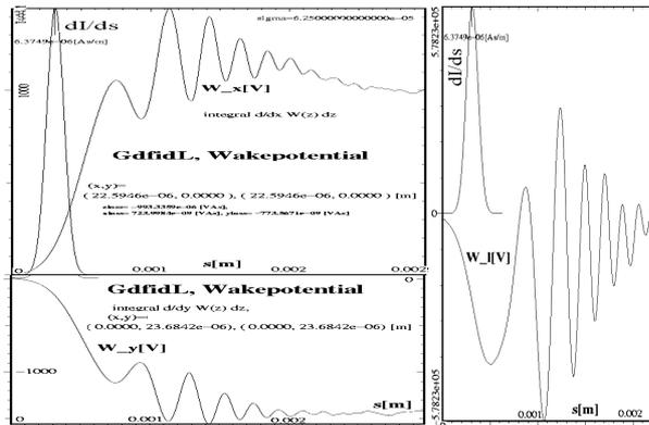
Figure 3: Short-range transverse (on the left) and longitudinal (on the right) wake-functions in 7-cell structure for  $\sigma = 63\mu\text{m}$  and  $q=4nC$ .
