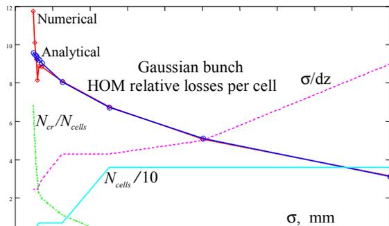
Figure 4: Monopole HOM energy losses related to fundamental mode loss per cell vs rms bunch length  $\sigma$ .
