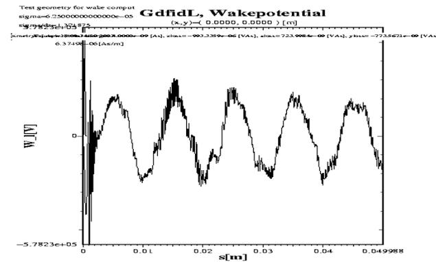
Figure 2: Longitudinal wake-function at  $\sigma = 62.5\mu\text{m}$ .
