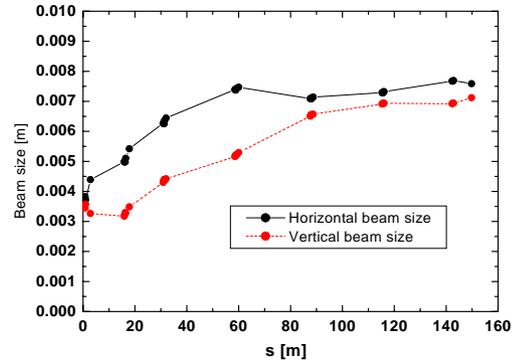
Figure 1: Beam sizes in the optics of the present 2.5 GeV linac.
