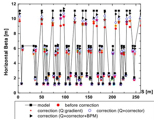
Figure 2: Horizontal beta-functions in the present 2.5 GeV storage ring
