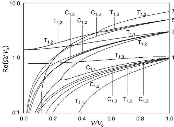
Figure 1: The real part of  $\Omega/\nu_o$  for the first sixteen  $m = 1$  modes versus  $\nu/\nu_o$  for  $ka = 1.0, b/a = 1.5,$  and  $Z = 0$ .
