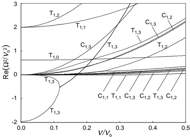
Figure 2: The real part of  $\Omega^2/\nu_o^2$  for the first sixteen  $m = 1$  modes as a function of  $\nu/\nu_o$  in the high-intensity region for  $ka = 1.0, b/a = 1.5,$  and  $Z = 0$ .
