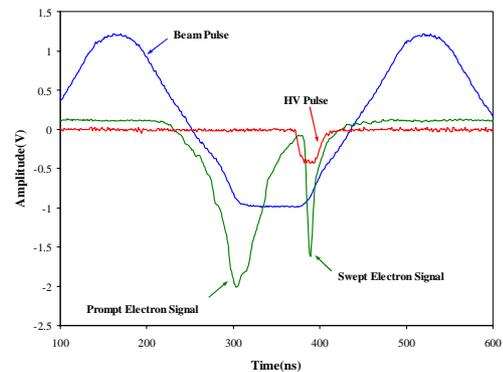
Figure 1. Swept electron signal from ESD plotted in time relationship to the HV and beam pulses.
