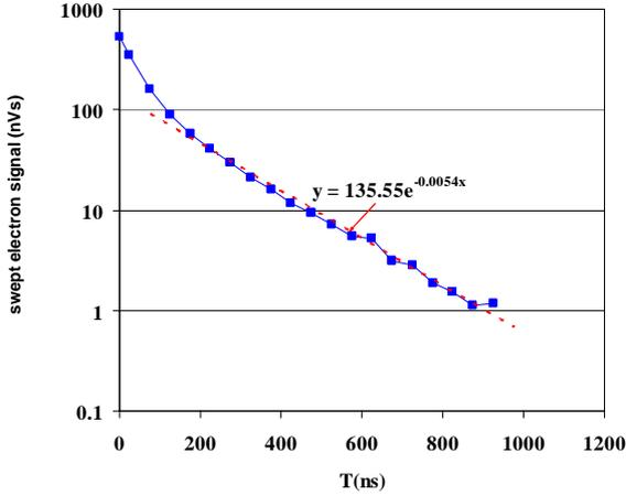
Figure 3. Swept electron signal (integral of pulse) plotted as a function of time after the end of the beam pulse.
