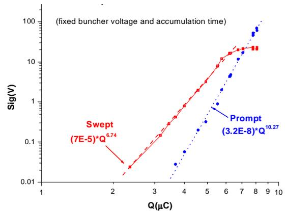
Figure 2. Prompt electron and “swept” electron signal amplitudes plotted as a function of stored beam intensity.
