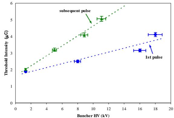
Figure 5. Plots of the instability threshold curves for the 1st pulse after a several minute wait and for the subsequent pulses for a small emittance beam in PSR.
