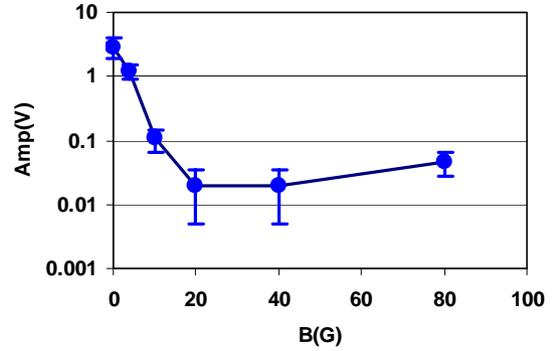
Figure 4. Effect of a weak solenoid field on the prompt electron peak amplitude.
