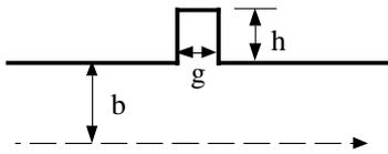
Figure 4: Sketch of a small cavity as a part of bellows, where  $b=40 \text{ mm}$ ,  $g=2 \text{ mm}$  and  $h=8 \text{ mm}$ . Note that a circular chamber is assumed instead of the actual racetrack type.
