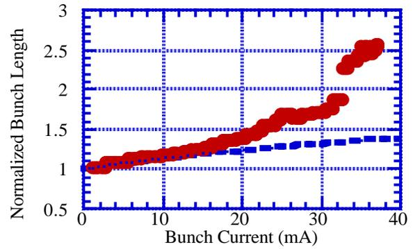
Figure 2: Normalized bunch length vs. bunch current for the new chamber measured in 2002 at 2.5 GeV. The dashed line is the calculated bunch length, assuming that the impedance is  $0.25 \Omega$ .  $\sigma_0=10.5$  mm.
