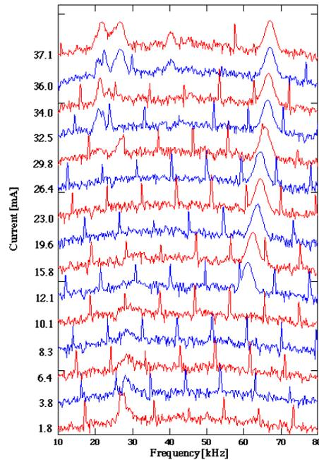
Figure 3: Sideband spectra for various bunch currents. The horizontal scale is frequency and the vertical scale is the bunch current. The spikes are the horizontal oscillation due to an injection error.  $f_s=28$  kHz.
