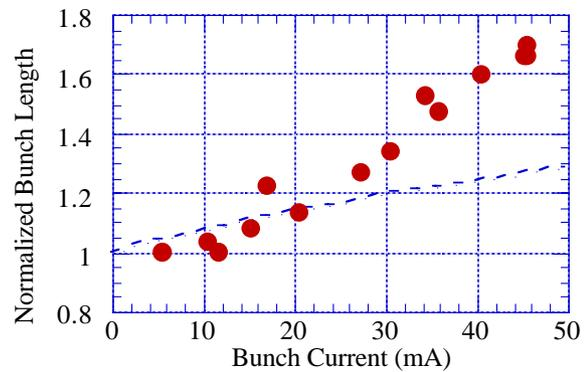
Figure 6: Normalized bunch length at a energy of  $3.0 \text{ GeV}$ . The dots are the measured bunch length; the dashed line is the calculated bunch length, assuming that the impedance is  $0.25 \Omega$ .  $\sigma_0=11.3 \text{ mm}$ .
