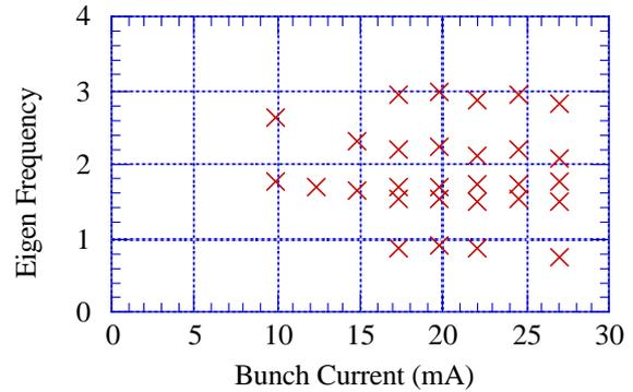
Figure 5: Imaginary part of eigenvalues normalized by synchrotron frequency as a function of the bunch current for the impedance of the new chamber.  $\sigma_0=8.75 \text{ mm}$ . Values for  $\text{Re}/\text{Damp} > 0.001$  are plotted.
