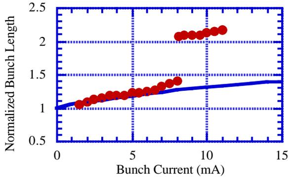
Figure 1: Bunch length normalized by the natural bunch length as a function of the bunch current for an old chamber measured in 1998 at 2.5 GeV. Dots are measured one and line is calculated bunch length based on the potential well.  $\sigma_0=12.2$  mm.
