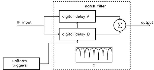
Figure 3: The digital notch filter.
