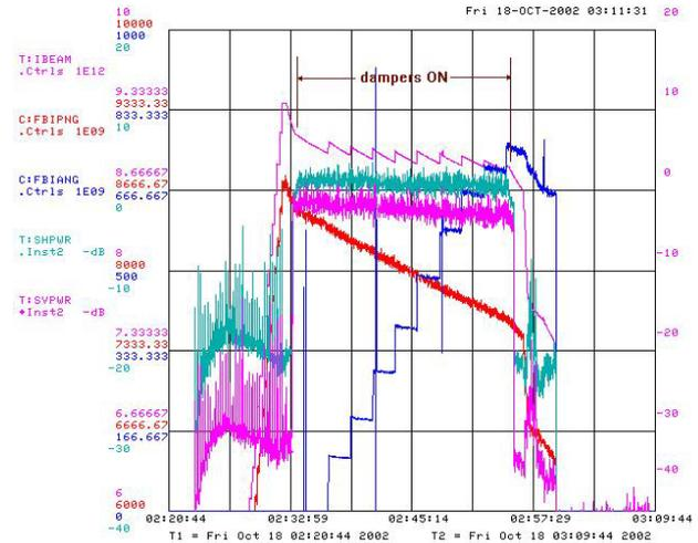
Figure 7: This plot shows the damper in action. Total beam current is T:IBEAM (the sawtooth shape comes from pbars being injected). C:FBIANG shows the increase in pbar current as they are being injected. C:FBIPNG is the proton beam current only. T:SHPWR and T:SVPWR are the horizontal and vertical Schottky powers which rise up by about 30 dB when the dampers are turned on.
