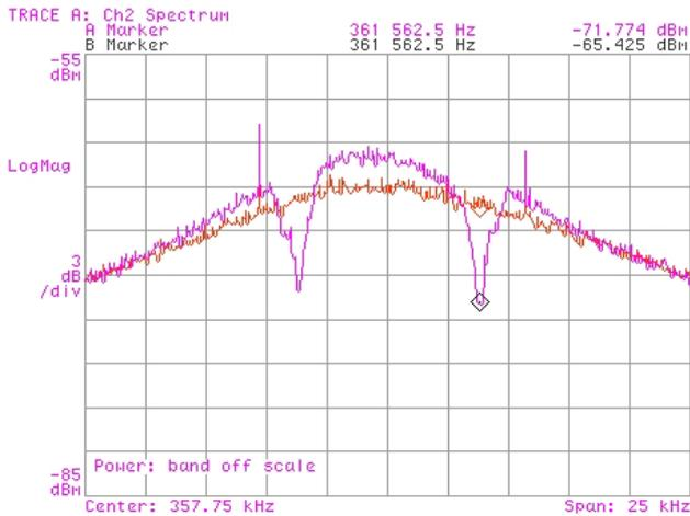
Figure 6: The suppression of the horizontal tune sidebands (purple curve) when the loop is closed compared to the red curve when it is open.
