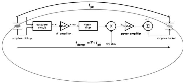
Figure 1: This is a block diagram which shows the overall setup of the transverse damper system. Note that the signal of the bunch which is detected at the stripline pickup is applied approximately one turn later to the same bunch at the stripline kicker. Each block is expanded further in Figures 2
