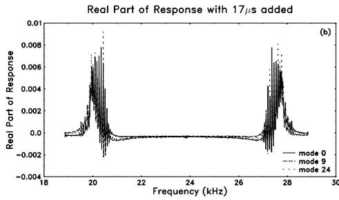
Figure 5: This graph shows real part of the response after adding  $17 \mu s$  to the digital delay. To get the real part of the response to be negative, we have to multiply by  $-1$  in the electronics. We have superimposed three graphs on top of each other by shifting the frequency of mode 9 by  $-9f_r$  and mode 24 by  $-24f_r$ .
