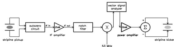
Figure 4: The loop is broken just downstream w.r.t. mixer and a vector signal analyzer (VSA) is connected there.
