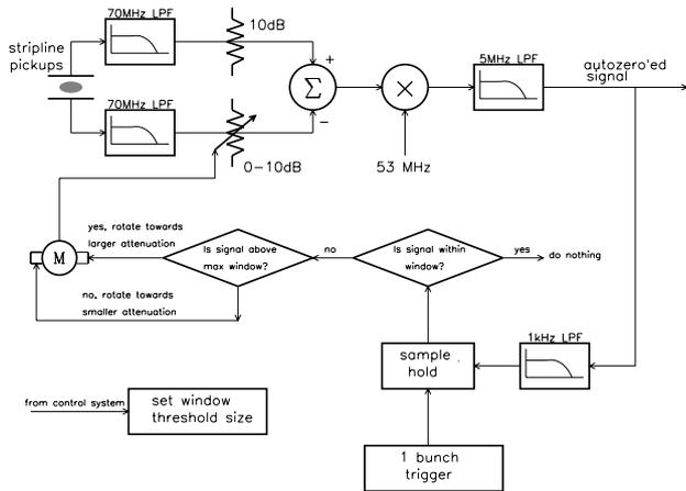
Figure 2: This figure shows the block diagram of the autozero circuit.
