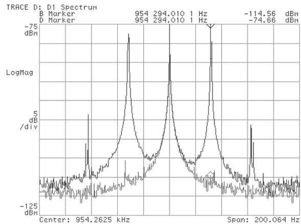
Figure 7: When we closed the loop at 980GeV, we excited the beam by anti-damping it. Then we turned on damping and clearly the synchrotron lines of mode 20 were damped.
