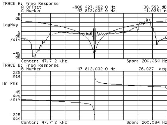
Figure 4: With both delays in the loop, we get notches near the revolution harmonics. The uncorrected imaginary response with one digital delay is superimposed for reference.
