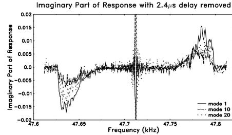
Figure 3: This graph shows the imaginary part of the response of modes 1, 10 and 20 after the delay is corrected. We have superimposed all the three graphs on top of each other by shifting the frequency of mode 10 by  $-10f_0$  and mode 20 by  $-20f_0$ .
