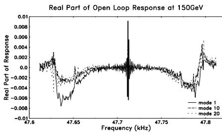
Figure 5: This graph show the real part of the open loop response of modes 1, 10 and 20 at 150 GeV. We have superimposed all the three graphs on top of each other by shifting the frequency of mode 10 by  $-10f_0$  and mode 20 by  $-20f_0$ .
