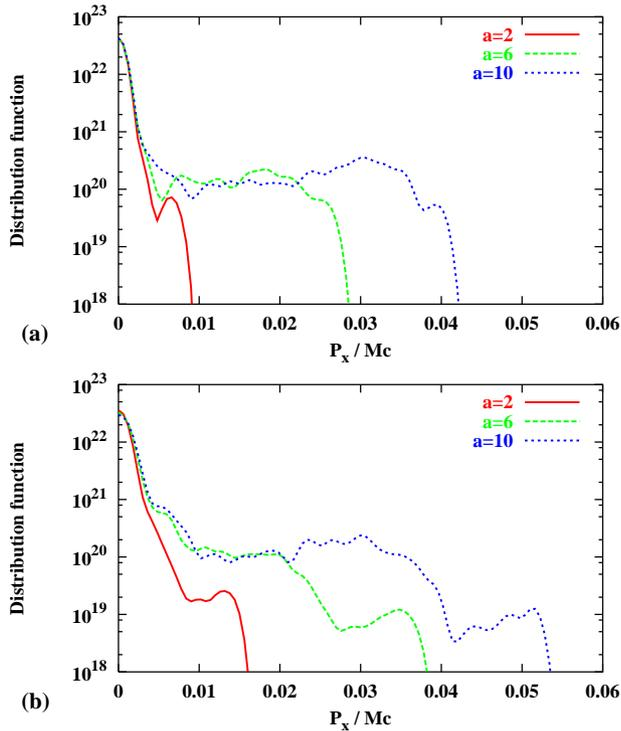
Figure 4: Momentum distribution functions of the accelerated ions for different laser intensities (a) without preplasmas and (b) with an exponential-profiled preplasma for  $n_1 = 0.9n_c$ . The profiles are measured at  $t = 247$  fs.
