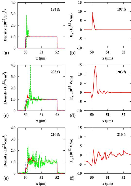
Figure 1: Shown are the profiles of the ion (solid) and electron (dashed) densities [(a), (c), and (e)] and the longitudinal electric field [(b), (d), and (f)] at different time. The dotted line in the density profiles shows the initial plasma profile. Simulation parameters are  $a = 10$ ,  $\tau_L = 10$  fs, and  $n_e = 9 n_c$ .
