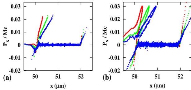
Figure 3: Momentum-position phase space for the cases of (a)  $n_1 = 10^{-3}n_c$  and (b)  $n_1 = 0.9n_c$  at  $t = 253$  fs, 287 fs, and 320 fs. Simulation parameters are  $a = 5$ ,  $\tau_L = 10$  fs.
