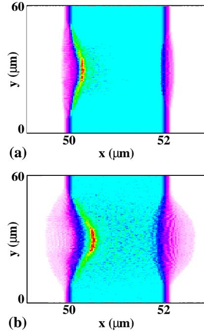
Figure 2: Density profile of the ions at (a)  $t = 239$  fs and (b)  $t = 292$  fs. Simulation parameters are  $a = 5$ ,  $\tau_L = 10$  fs, and  $n_e = 9 n_c$ .
