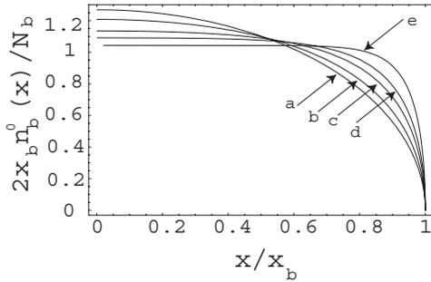
Figure 1: Plots of the normalized density profile  $2x_b n_b^0(x)/N_b$  versus  $x/x_b$  for different values of the normalized beam intensity  $s_b$  corresponding to (a)  $s_b = 0.2$ , (b)  $s_b = 0.9$ , (c)  $s_b = 0.99$ , (d)  $s_b = 0.999$ , (e)  $s_b = 0.999999$ .
