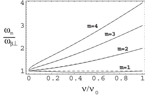
Figure 2: Plots of the normalized mode frequencies  $\omega_m/\omega_{\beta\perp}$  versus the on-axis ( $x = 0$ ) tune depression  $\nu/\nu_0 = (1 - s_b)^{1/2}$  for several values of mode numbers  $m = 1, 2, 3, 4$ . The dotted curves are the numerical solutions of the eigenvalue equation (27); the solid curves are the solutions obtained in the WKB approximation [Eq. (32)].
